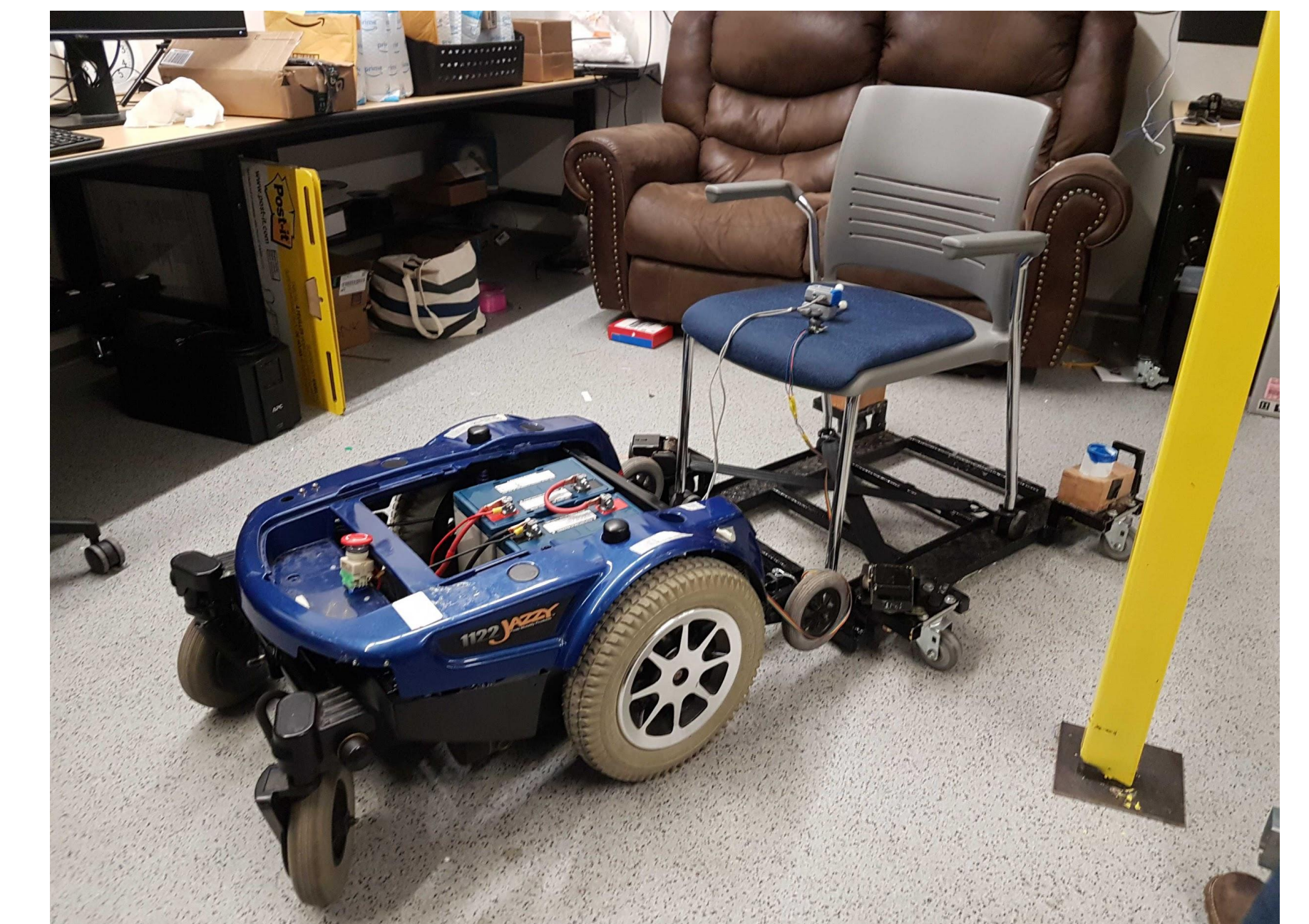
The final platform without the head switches mounted.
